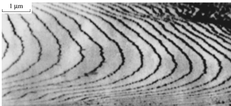
Fig. 2. Representative image of the stepped Si(111) surface exposed to the oxygen atmosphere at a pressure below P_{\text{crit}} . Monatomic steps moved from left to right.
